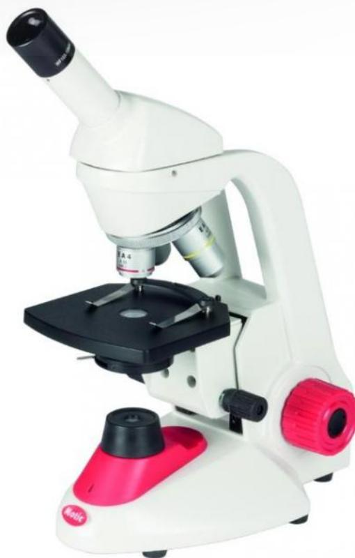
Microscope MOTIC RED100 monocular désaxé 4X/10X/40X LED
