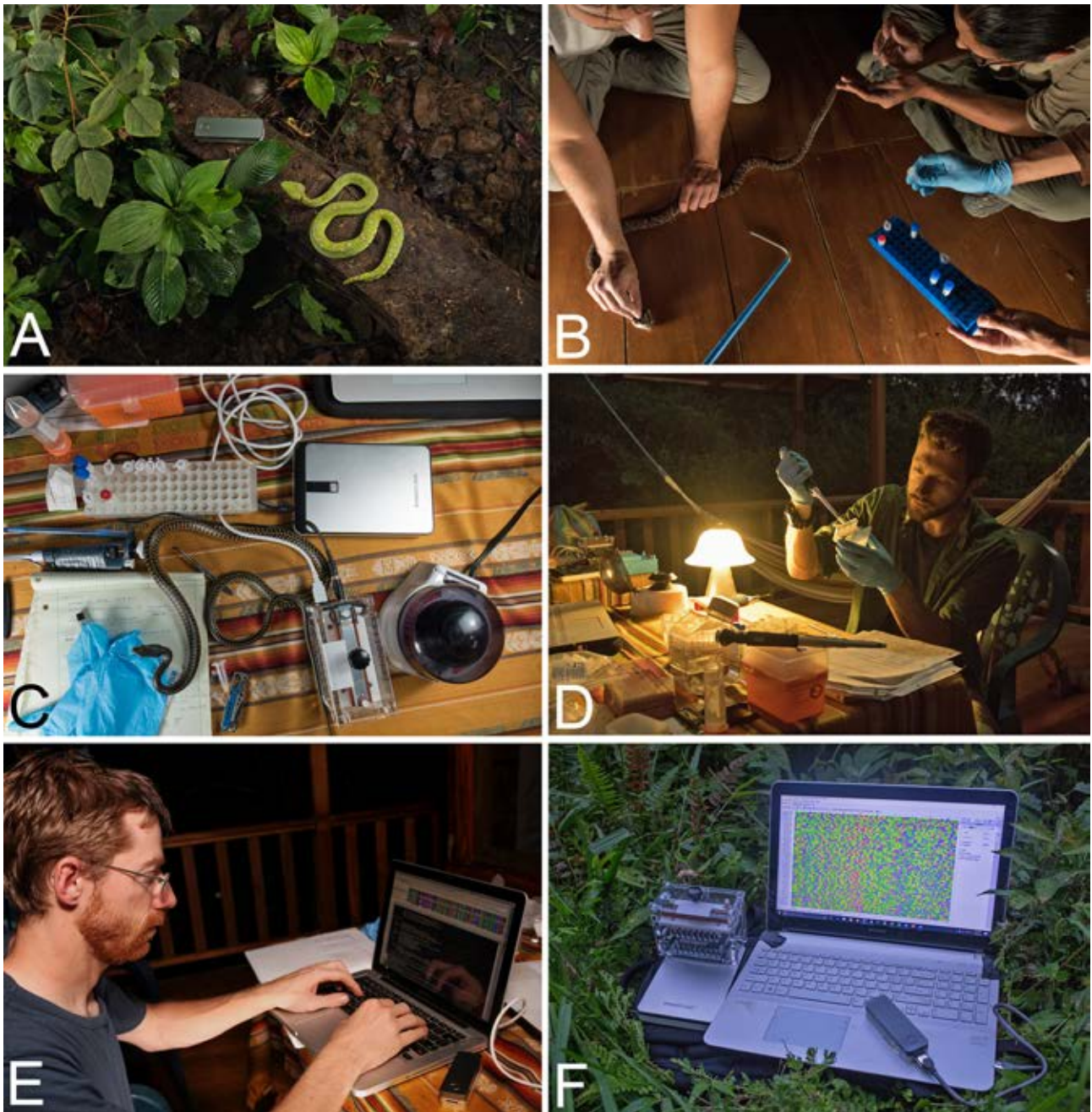
Figure 1: Process of nanopore sequencing in the Ecuadorian Chocó rainforest. (A) Sampling endemic fauna; eyelash pitviper next to MinION. (B) Extraction of blood or tissue samples. (C) DNA extraction using the DNeasy kit and benchtop centrifuge, and PCR amplification with the MiniPCR. (D) Oxford nanopore library preparation of DNA barcodes. (E) Bioinformatic processing of nanopore data in the field. (F) Primary equipment used in portable sequencing, left to right: MiniPCR sitting atop Poweradd external battery, MinION plugged into a Windows laptop displaying Geneious Pro software of raw nanopore data.
