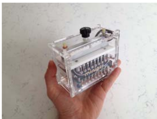
Fig. 1. MiniPCR™ mini8 Thermal Cycler (source: http://www.minipcr.com )
